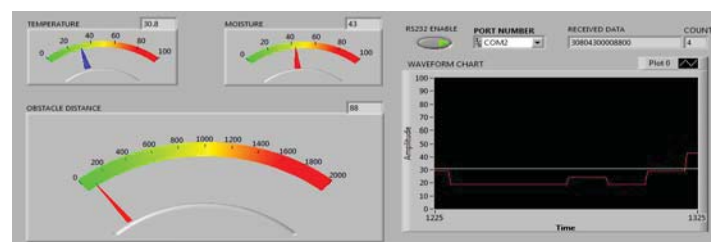
Fig 3.3 Temperature and Moisture detection
