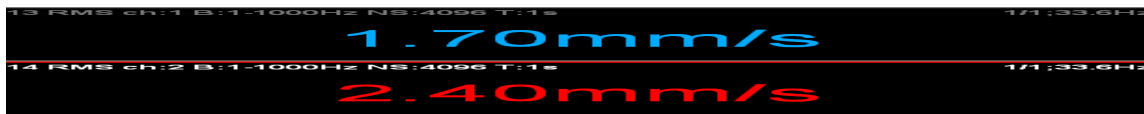
Figure 21. Experimental frequency domain vibration reading of channel 1 & 2 of without damper and without unbalanced mass.
