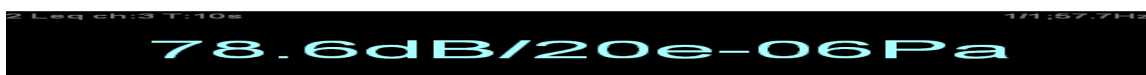
Figure 50. Experimental noise level reading of channel 1 & 2 of with Cork felt damper and with unbalanced mass.
