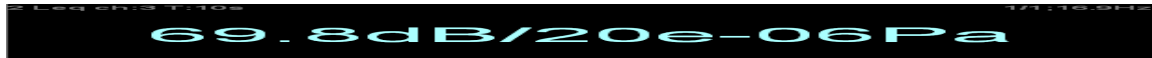
Figure 53. Experimental noise level reading of channel 1 & 2 of with Cork felt damper and without unbalanced mass.
