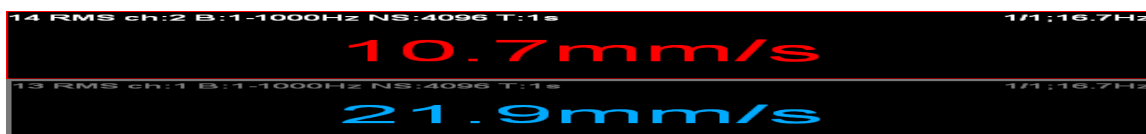
Figure 18. Experimental frequency domain vibration reading of channel 1 & 2 of without damper and with unbalanced mass
