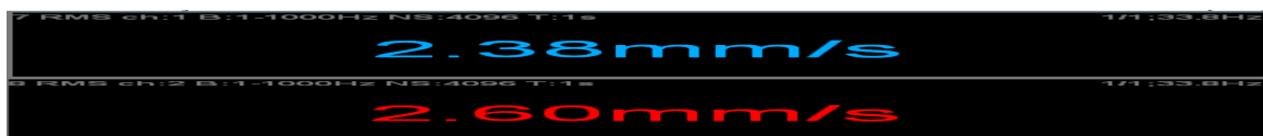
Figure 55. Experimental frequency domain channel 1 & 2 of with Cork felt damper and without unbalanced mass.
