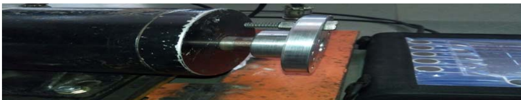
Figure 10. Slotted disc with unbalanced mass used in Experiment.
