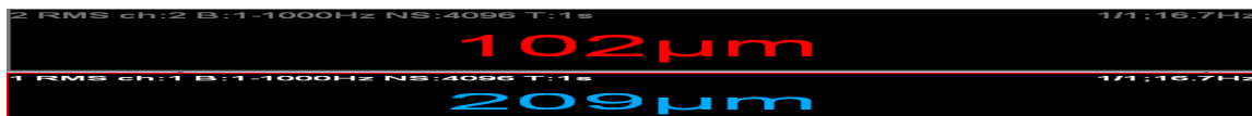
Figure 17. Experimental time domain vibration reading of channel 1 & 2 of without damper and with unbalanced mass.
