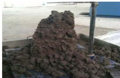
Fig 5.10 Slump Cone Test
