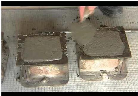
Fig.5.4 Mortar cube
