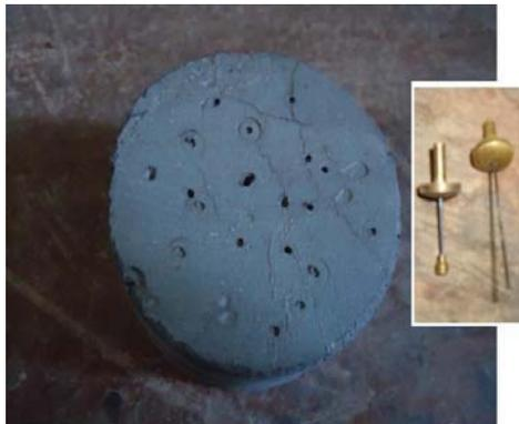
Fig. 5.2 Tested Cement Cube Along With Final & Initial Setting Time
