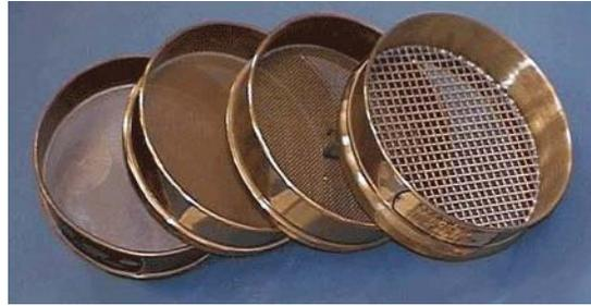
Fig.5.5 Fine aggregate Sieves
