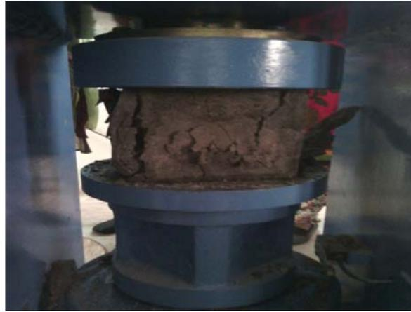
Fig 5.12 Compression Test On Cube Element
