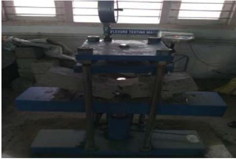
Fig 5.14 Flexural Test Test On Beam Element
