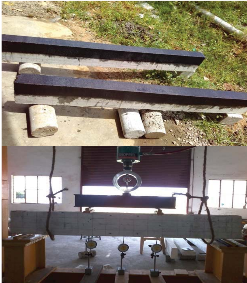
Figure 5. control beam testing Table 4. Deflection test on Specimen
