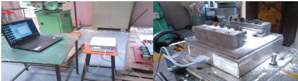
Fig 1. Machining of GFRP laminate plate is properly fixed in machining center by special designed fixture with data acquisition laptop attachment
