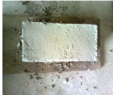
Fig.8 Casted brick kept for Air curing
