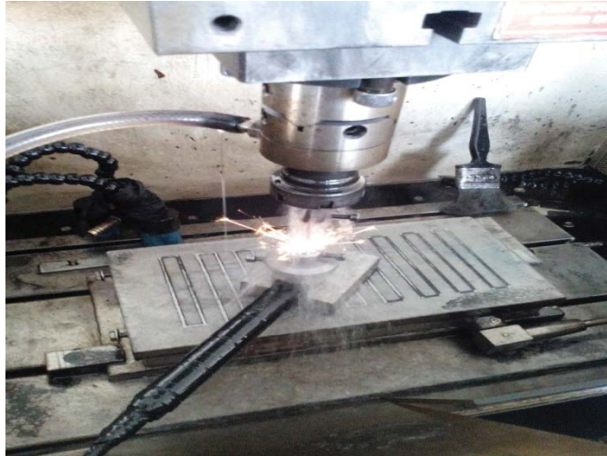
Fig. 2: Working set up of vibration assisted EDM
