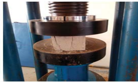
fig.4.5 compressive strength on brick & brick masonry
