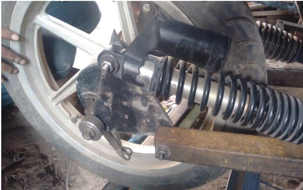
Fig 3.3. Setup of modified horizontal dual suspension system (right hand side)
