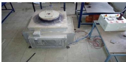
Fig 2. Stir casting furnace used for preparation of AMCs.
