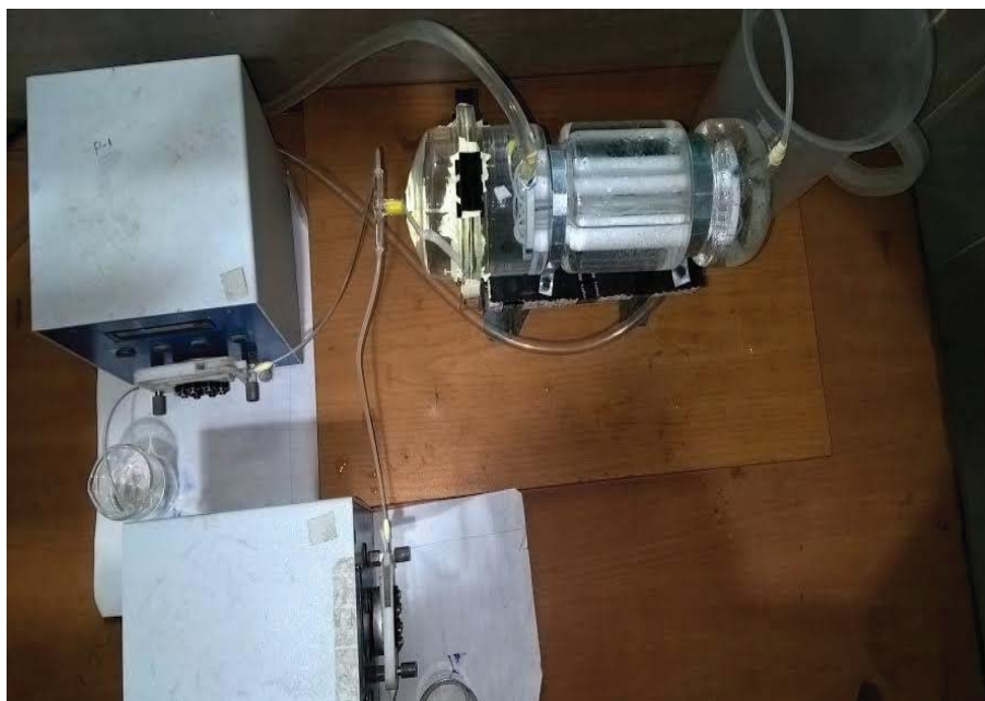
Fig 2: MilliReactor – Experimental Device with Peristaltic Pumps
