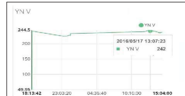
Fig. 7.6 Average LN Voltage monitored on 17/05/2016 at 12:55
