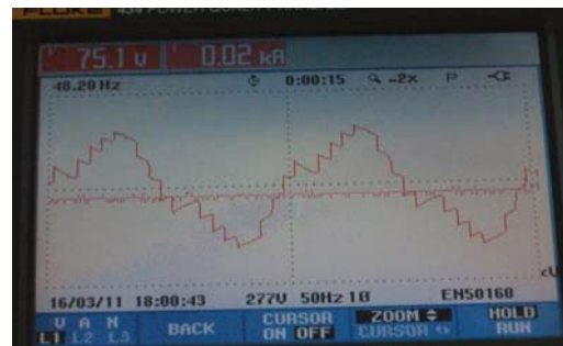
Fig.19. Output Voltage with 1kW R load
