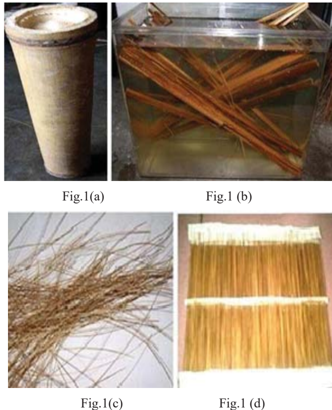
Figure.1. Process of bamboo fibers - (a) bamboo cylindrical portion of culm,(b) strip soaked in to water , (c)Extract bamboo fibers, (d) bamboo mat
