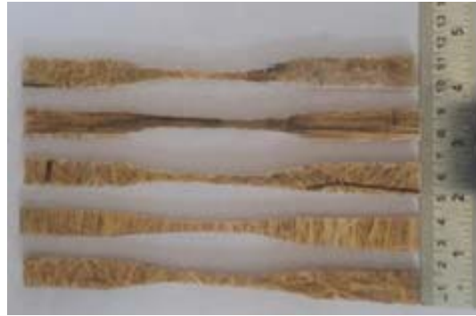
Figure. 3. Tensile Specimen as per ASTM standards
