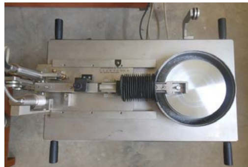
Figure1: DUCOM wear and friction monitor pin on disc wear testing machine
