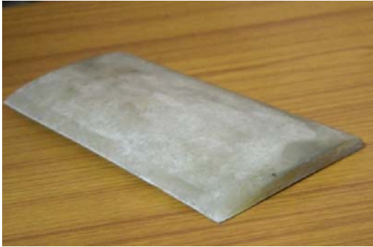
Figure 10. Wing fabricated with FRCM
