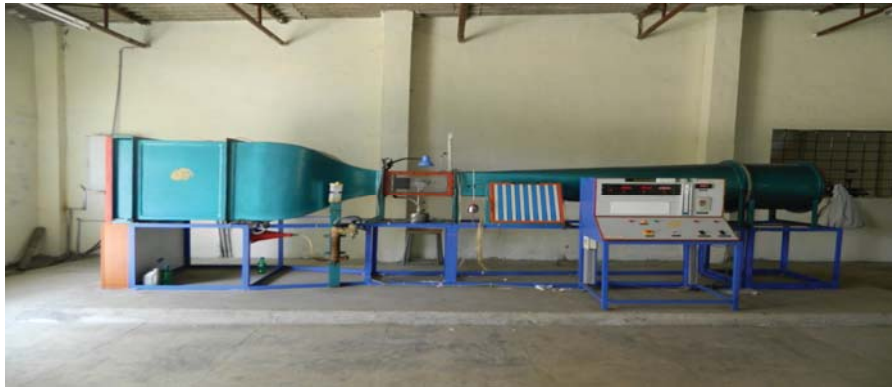
Figure 12. Low Speed Subsonic Wind Tunnel
