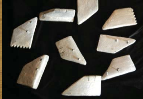
Figure 11. Winglets modelled with FRCM
