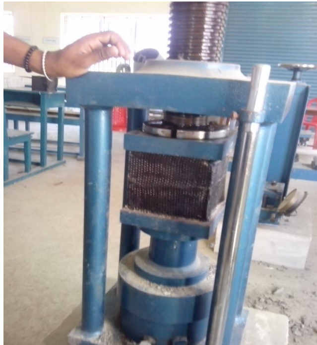
Figure 5. Compressive Strength Testing on U 4
