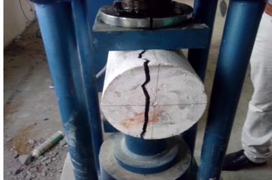
Figure 8. Split tensile strength on U 1 and Control
