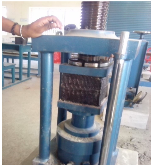
Figure 5. Compressive Strength Testing on U 4
