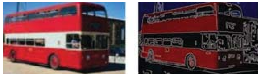
Figure.2. (a) Original RGB image (b) RGB image with edge information (edges extracted from Y matrix)
