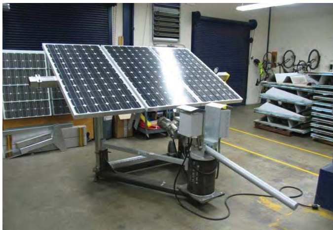
Power Tracker test rig in Power Light engineering shop
