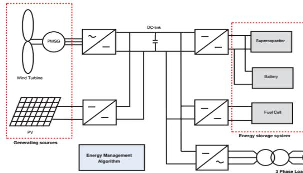
Fig.1. Block schematic of DC microgrid
