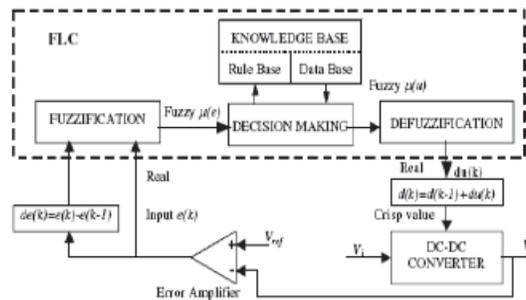
Fig.3. Block diagram of the Fuzzy Logic Controller (FLC) for dc-dc converters
