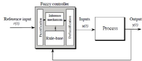
Fig.2. General Structure of the fuzzy logic controller on closed-loop system
