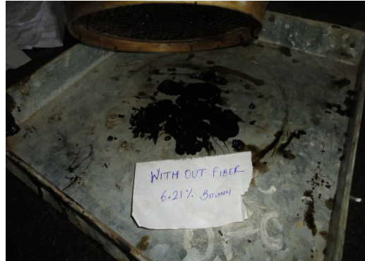
Fig. 2. Drainage of bitumen from mix -without fibre
