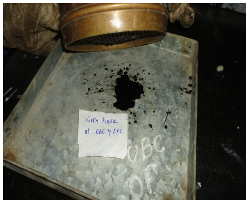
Fig. 3. Drainage of bitumen from mix -with fibre at OBC and OFC
