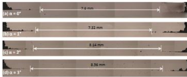
Fig. 5. Effect of tilt angle on bonding interface. Process parameters: F = 5 \text{ kN} , \Omega = 2500 \text{ rpm} and v = 10.5 \text{ mm/s} .
