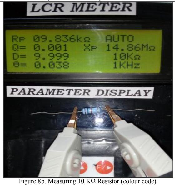
Figure 8b. Measuring 10 KΩ Resistor (colour code)
