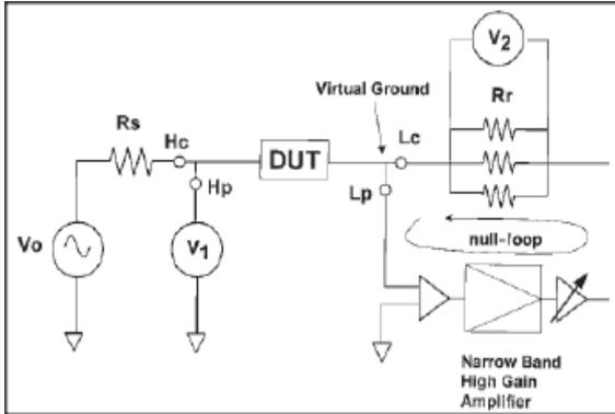
Figure 3. Circuit diagram of the Auto-Balancing
