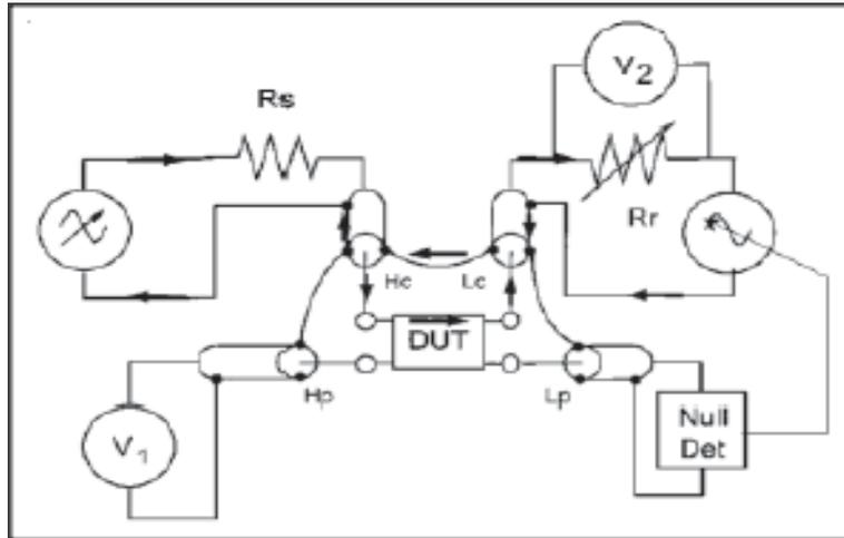
Figure 5. Combination of the Auto-Balancing-Bridge with the Four-Terminal-Pair configuration
