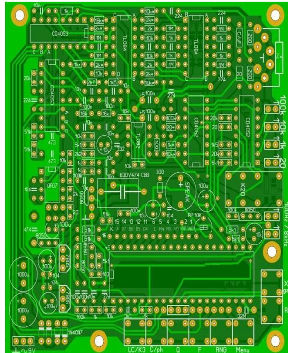
Figure 7b. Printer Circuit Board of LCR meter
