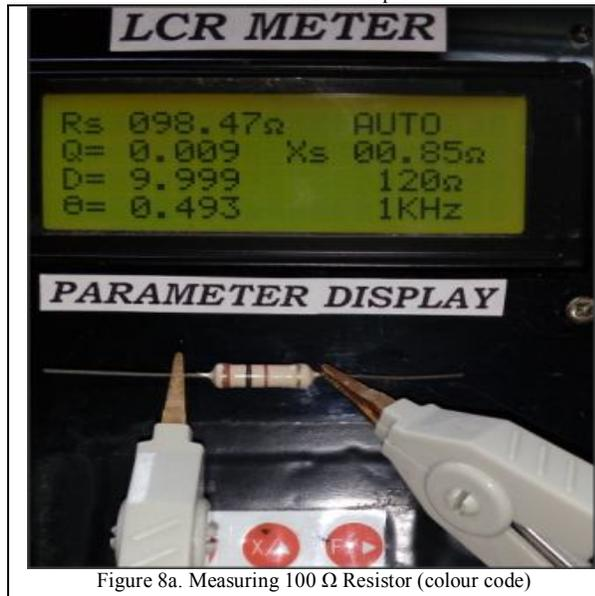
Figure 8a. Measuring 100 Ω Resistor (colour code)
