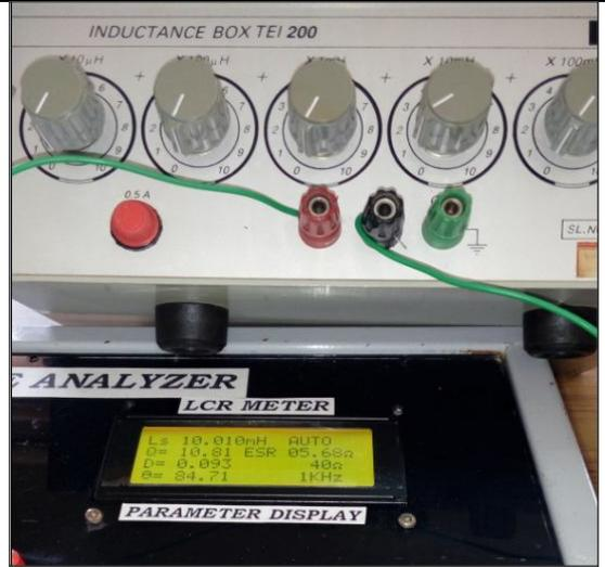
Figure 8d. Measuring 10 mH Inductor (box)
