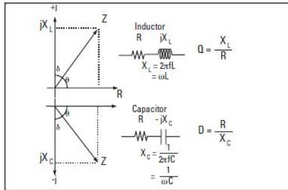
Figure 2. Capacitor and Inductor Parameters
