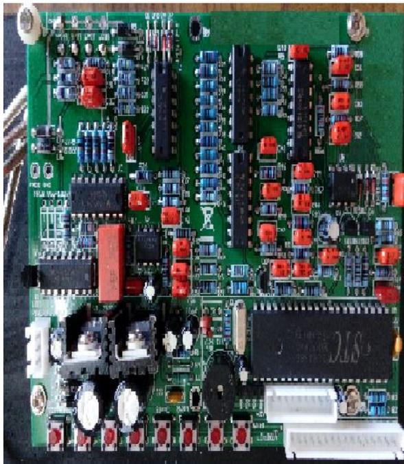
Figure 7c. Fabricated LCR meter
