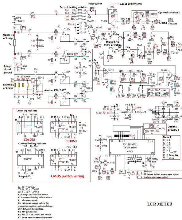
Figure 7a. Circuit diagram of the LCR meter
