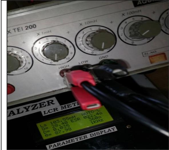
Figure 8c. Measuring 100 mH Inductor (box)
