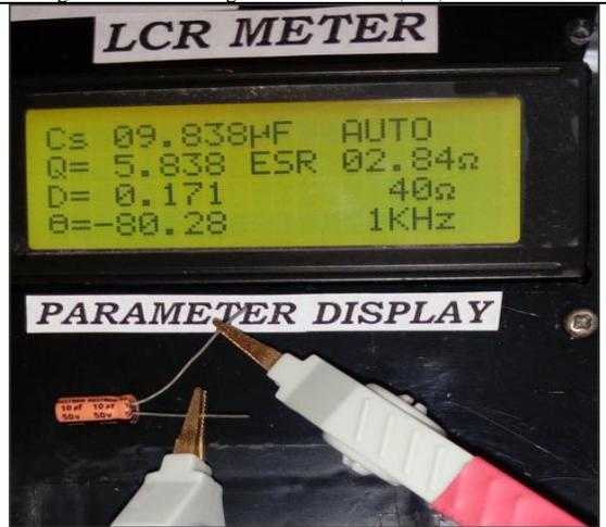
Figure 8f. Measuring 10 uFarads Capacitor
