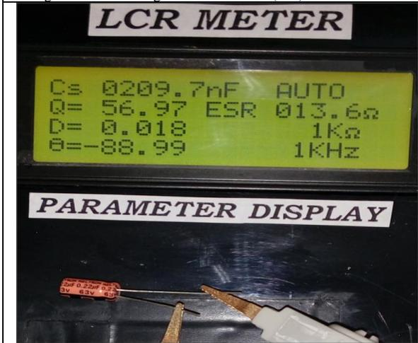
Figure 8e. Measuring 0.22 uFarads Capacitor
