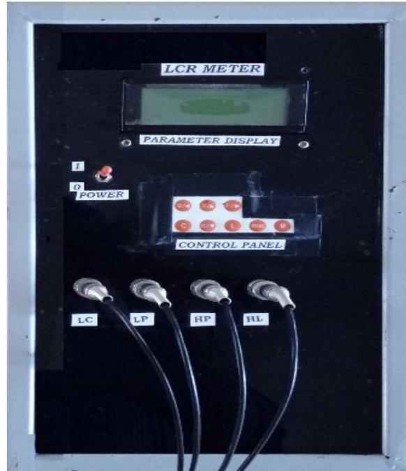
Figure 7d. Front panel of fabricated LCR meter
