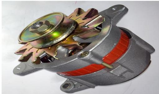
Fig. 2: Dc Alternator motor (Car)
