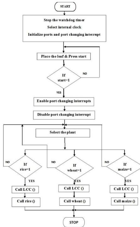
Fig.2.Flowchart for finding the nitrogen deficiency detector
