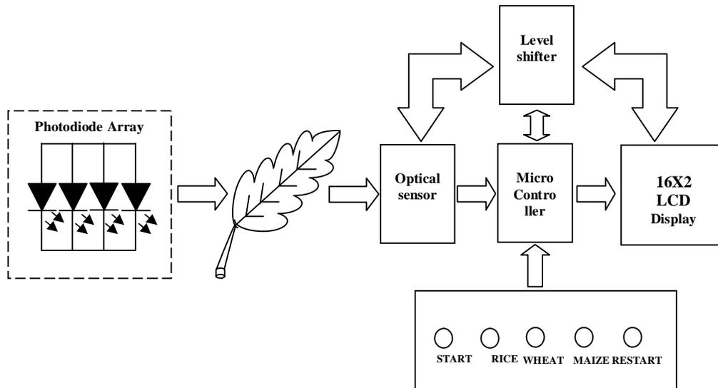
Fig.1 Block diagram for Nitrogen deficiency detector
