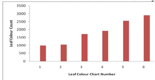
Fig.4. Calibration of TCS3200 without proper cover for rice plant
