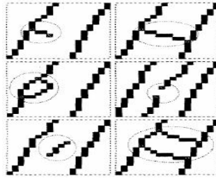
Figure 6. A. Spike, B. Bridge, C. Hole, D. Break, E. Spur F. Ladder
