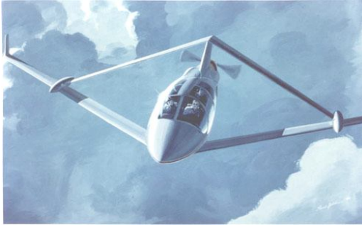
Fig 1 (c)Strut- braced system
