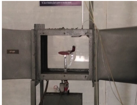
Fig.12. Wind Tunnel testing of C wing with 90°
