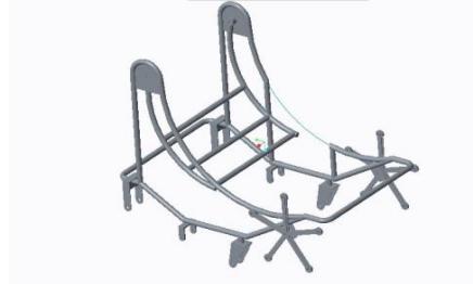
Figure 2. Isometric view of frame with planetary wheel chair
