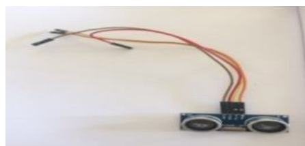
Figure 6. Ultrasonic module with wire
