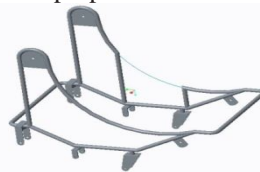
Figure 1. Isometric view of the frame (Design in CREO)
