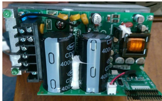
(b) Rectifier-Inverter Set
