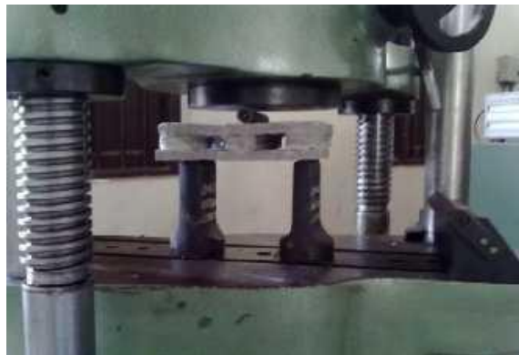
Fig 3. Flexural strength test on tile
