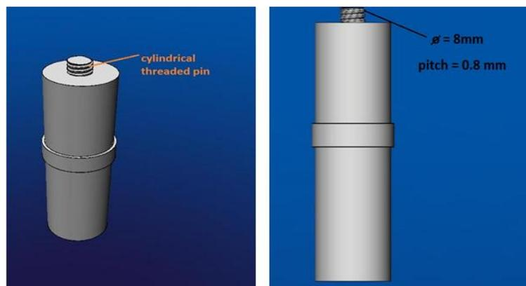
Figure2 Cylindrical threaded tool
