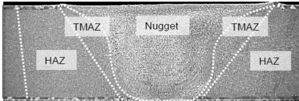
Figure3 Different type of zones in welded region – weld nugget, thermo mechanically affected zone (TMAZ), and heat affected zone (HAZ).
