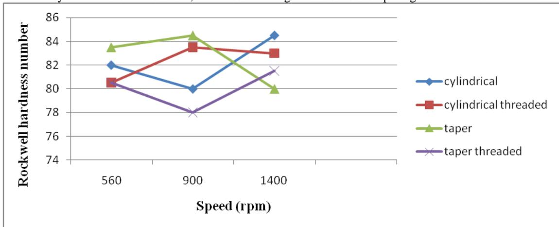
Figure 6 Rockwell Hardness of FSW Aluminum 7075 joints.
