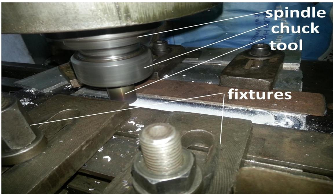
Figure1 Friction Stir Welding Setup
