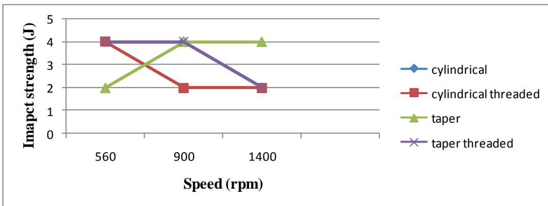
Figure 5 Impact Strength of FSW AA7075-T6 joints.
