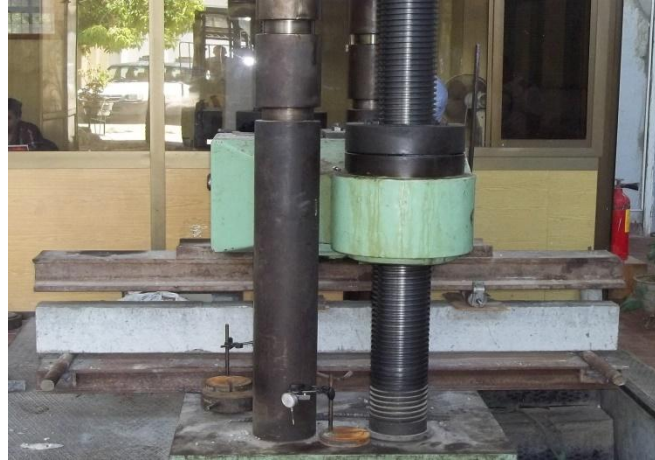
Figure 2. Flexure tests of concrete beams
