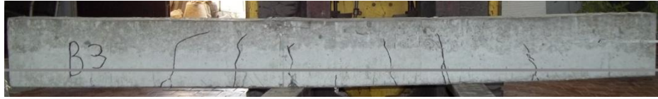
Figure 8. Crack Pattern of Beams B3
