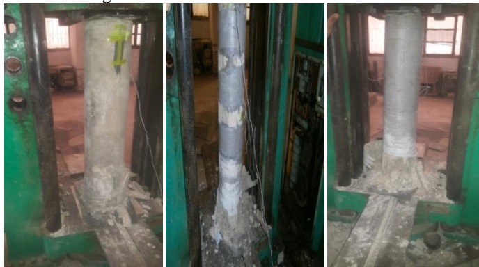
Figure 2. Test setup and shape of failure of circular specimens.
