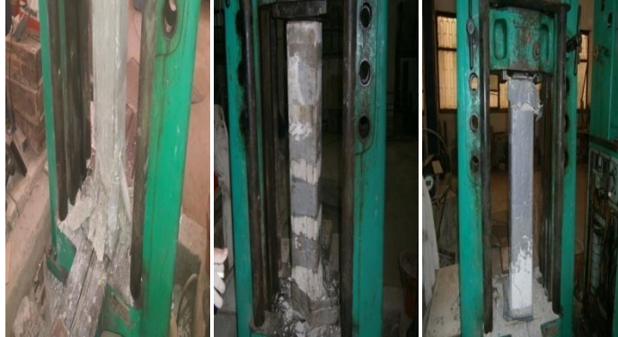
Figure 3. Test setup and shape of failure of square specimens.
