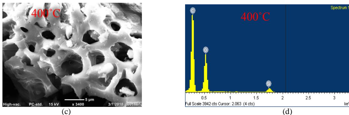
Figure 1. (a) SEM and EDX spectrom of rice husk biochar at 300 °C for 1h (b) SEM and EDX spectrom of rice husk biochar at 400 °C for 1h
