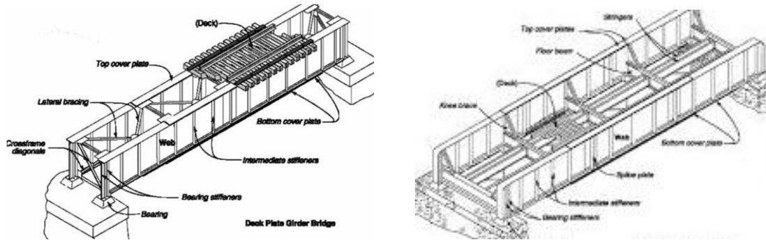
Figure 3. (a) deck type bridge (b) through type bridge
