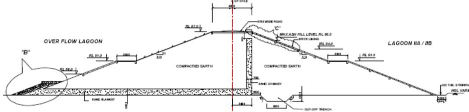
Figure 3 :Cross section of Starter Dyke at Tanda Thermal Power Project
