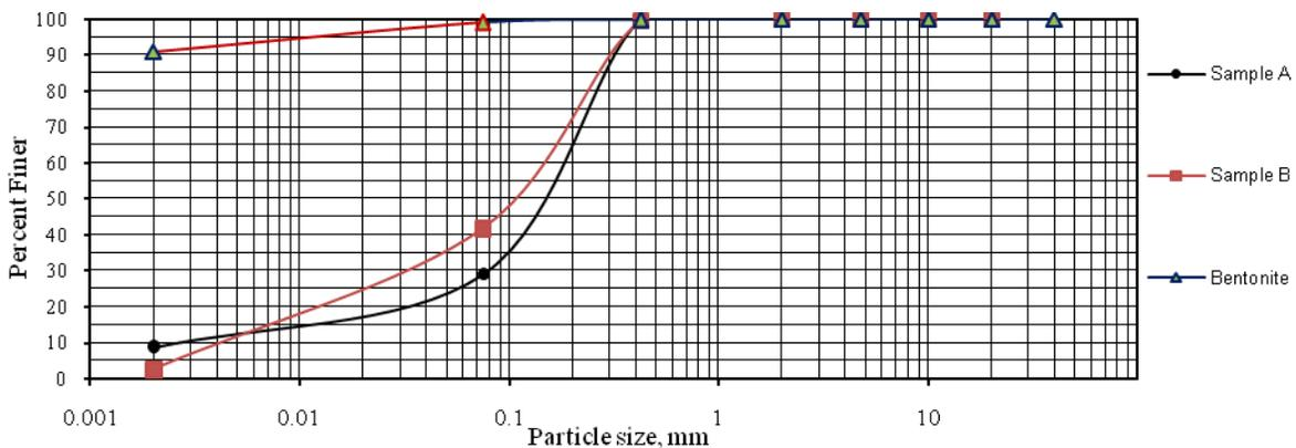
Figure 4: Grain Size distribution of Borrow Areas Soil and Bentonite
