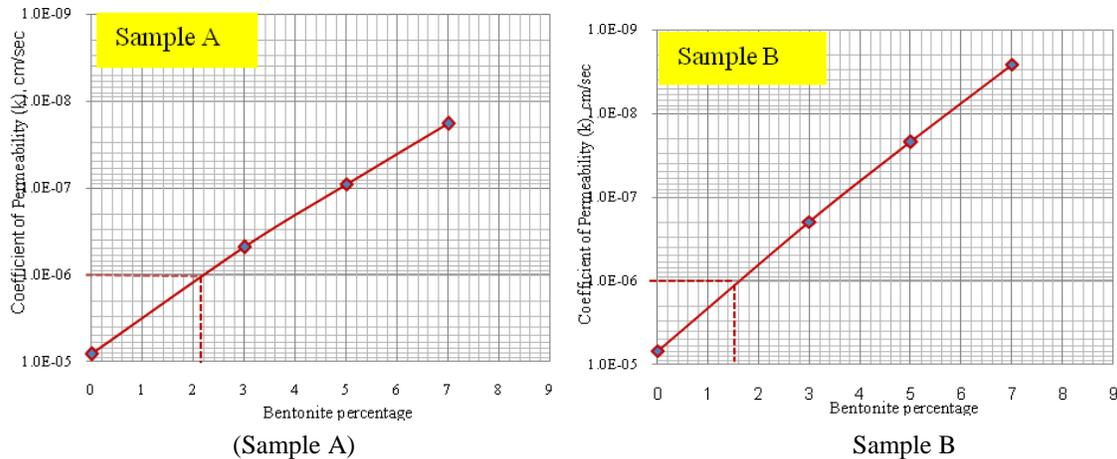
Figure 6: Coefficient of Permeability(k) Vs. Bentonite Percentage for Blended Soil Samples A and B
