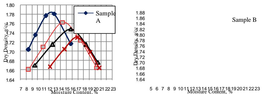
Figure 5: Standard Proctor Compaction Curves of Blended Soil Samples A and B
