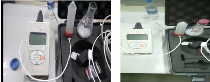
Fig 2 showing measurement of Thermal Conductivity
