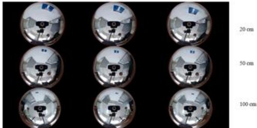
Figure 2. Example of the measurement performed for a Square panel to compute its Hu invariant moment vector in different distances and heights from the catadioptric camera
