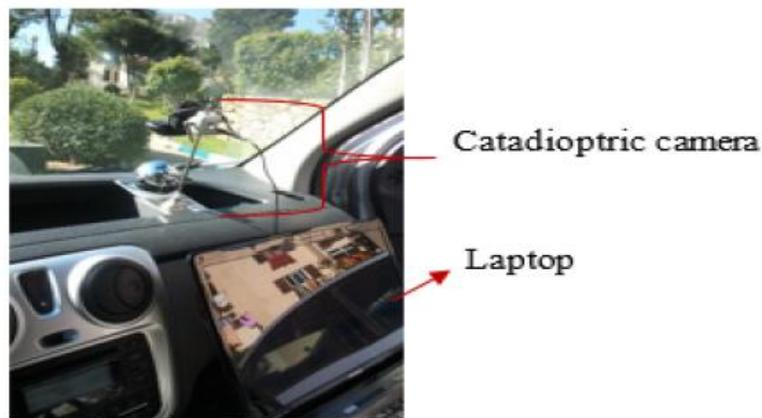
Figure 4. Catdioptric camera and laptop used in this work
