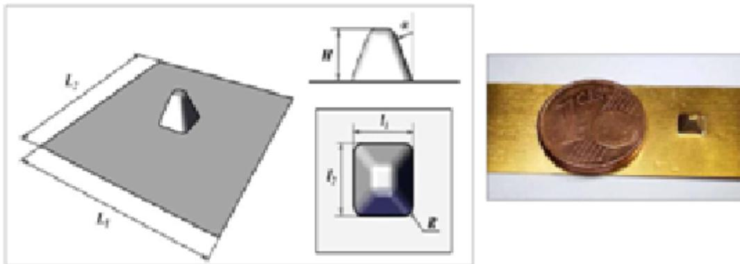
Figure2. (a) Geometry of pyramid (b) Sample of forming pyramid by ISF
