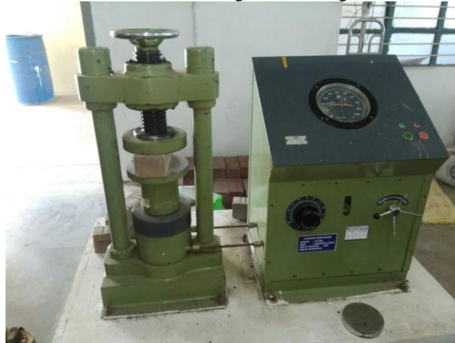
Figure.2 Compression test on bricks
