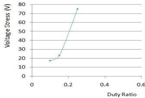
**Figure 13. Voltage stress versus duty cycle**
