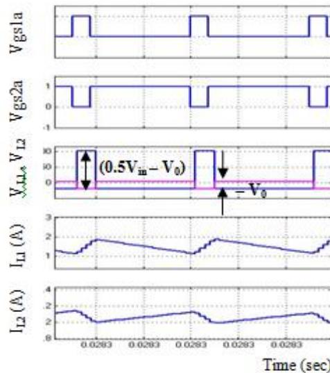
**Figure 5. Theoretical waveforms of the Converter.**
