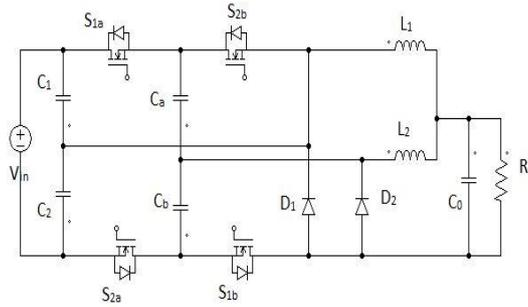
**Figure 3. Transformer less interleaved Buck Converter.**
