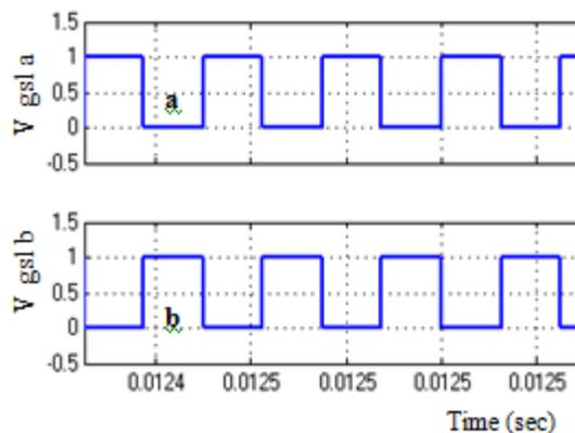
**Figure 9. Switching pulses to S<sub>1a</sub> and S<sub>2a</sub>**
