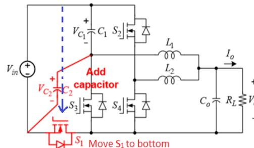
Figure 1. Deriving the Modified Series Capacitor Buck Converter [2].
