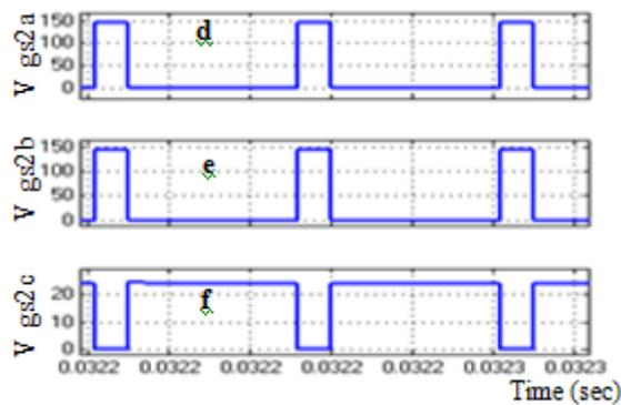
Figure 12. Voltage Stress across (a)  $S_{2a}$  (b)  $S_{2b}$  (c)  $S_{2c}$
