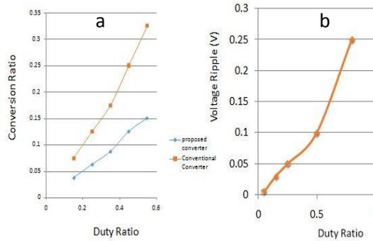
**Figure 12. Duty ratio Vs (a) Conversion Ratio (b) Voltage Ripple**
