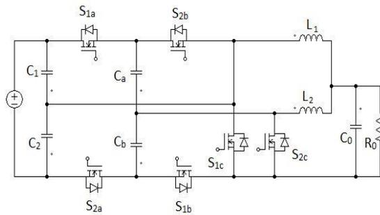
**Figure 4. Transformer less interleaved Buck Converter.**
