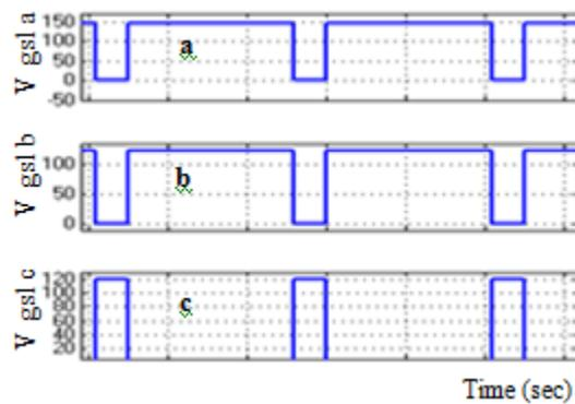
Figure 11. Voltage stress across (a)  $S_{1a}$  (b)  $S_{1b}$  (c)  $S_{1c}$
