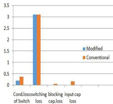
**Figure 14. Losses of modified converter**
