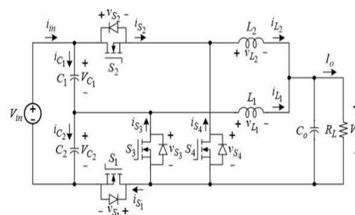
Figure 2. Modified Series Capacitor Buck Converter.
