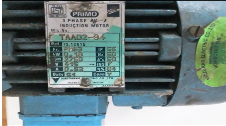
Figure 8: 3-phase induction motor rating specifications.
