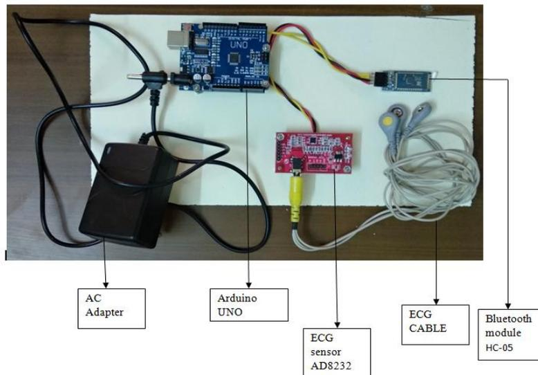
Figure.8 ECG monitoring system
