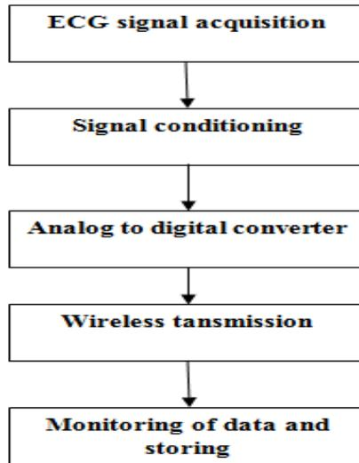
Figure 7. Acquisition of ECG using hardware component.
