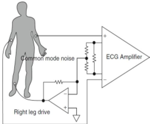
Figure 5. Right leg drive circuit
