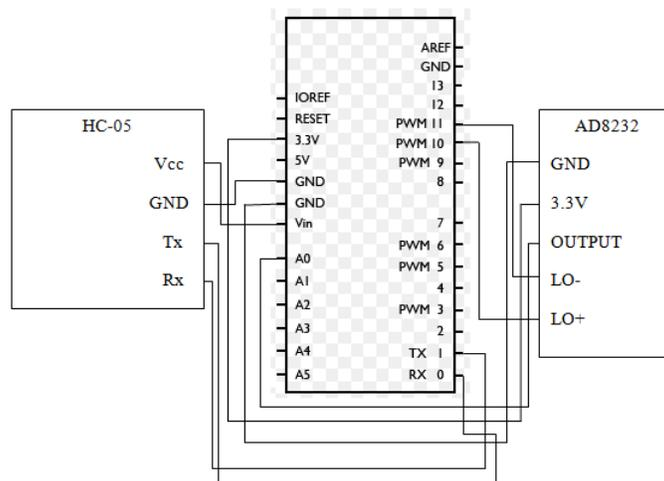
Figure 6. Circuit diagram for ECG signal acquisition system
