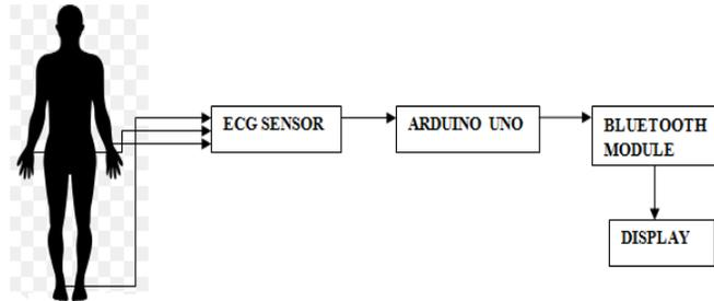
Figure 4. Architectural block diagram
