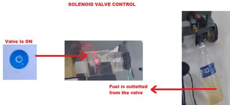
Figure 7: Solenoid valve control
