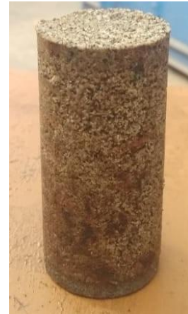
Figure 1: Microbially Treated Sand D_{50} = 0.257 mm Figure 2: Microbially Treated Sand D_{50} = 0.486 mm
