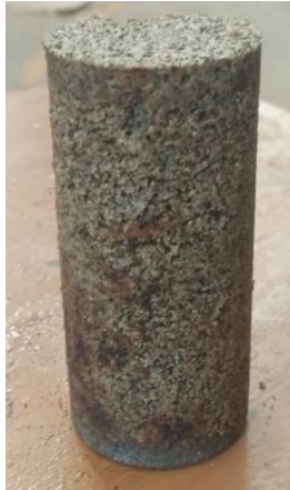
Figure 1: Microbially Treated Sand D_{50} = 0.257 mm Figure 2: Microbially Treated Sand D_{50} = 0.486 mm
