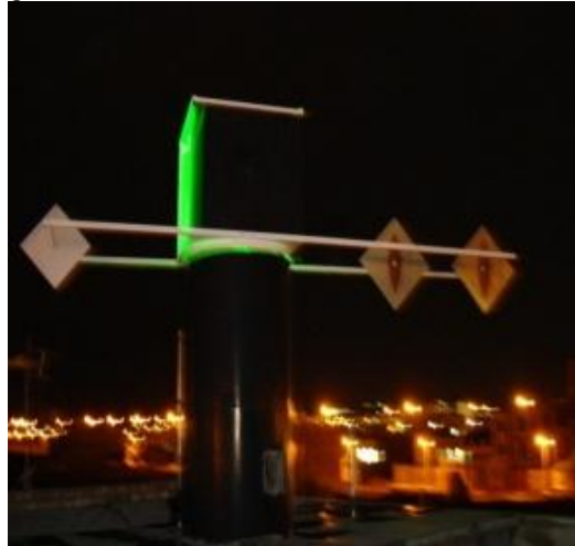
Fig.4 Tower unit of an evaporative cooling system which is aligned in the wind direction of wind
