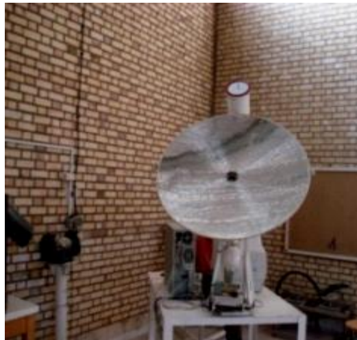
Fig.3 A non -integrated parabolic mirror (solar dish) and its intelligent navigator system
