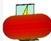
Fig .8. E-pattern of triangle antenna with horizontal nullifier
