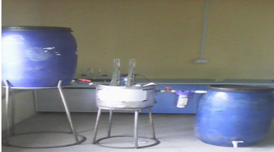
Plate I: Designed and Fabricated Bench Scale Water Treatment plant used in this study
