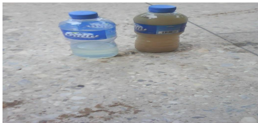
Plate V: Image of Treated Water via Fabricated Treatment Units Using Processed Balanites Aegyptiaca Seed Powder
