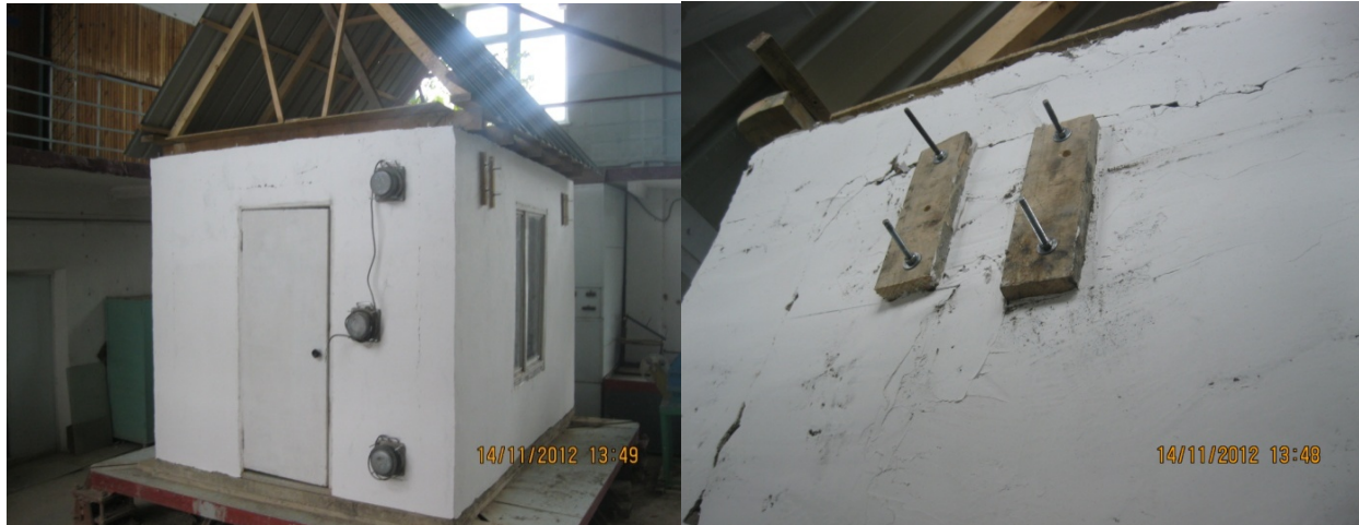
Fig 6. General view of the model house of «reinforced concrete frame» after the experiment
