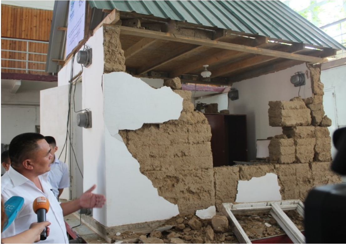
Fig1. General view of the model of the house «sokmo» after the experiment
