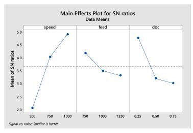
The experimental result show the average surface roughness low at higher speed and lower depth of cut. ANNOVA show the speed is the most influence parameters for surface roughness. Optimum parameters setting for surface roughness is
